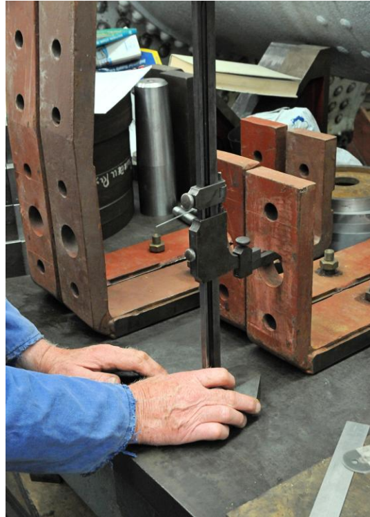
Ex-9F axle box guides for 84030's hind pony truck
