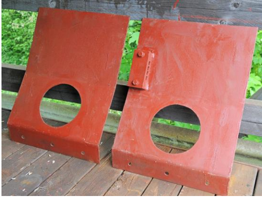
In-fill plating with leading sandbox filler openings
