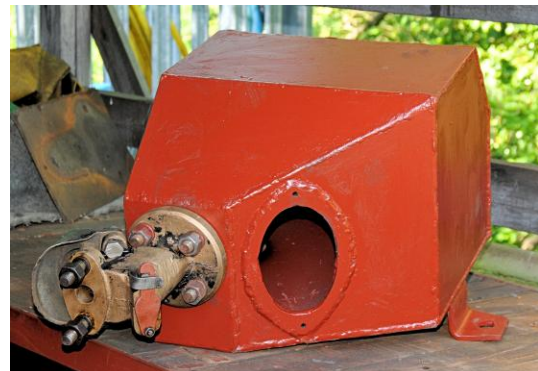
First of two hind sand-boxes nearing completion
