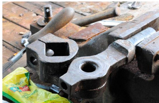
Restoring lubricator drive fittings
