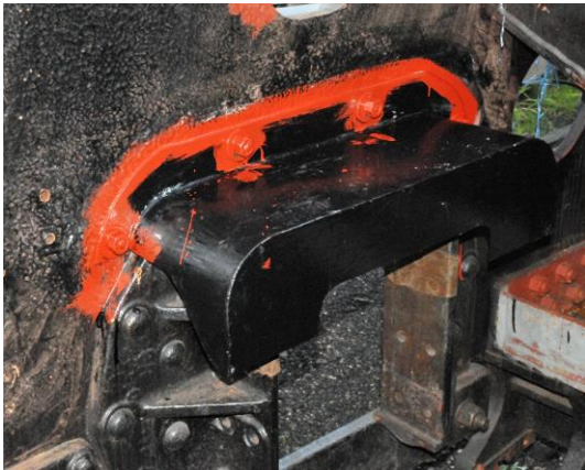
RHS trailing axle box shield in place.
