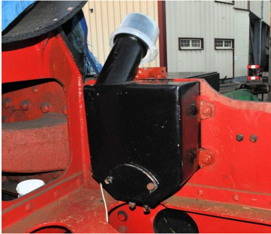
RHS front sandbox in place.
