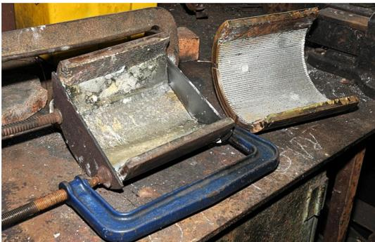
Re-metalling Coupled Wheel Axlebox Bearings
